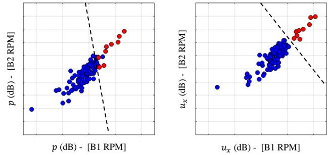
Figure 7. Linear classifier based on features extracted from two different RPM bands (B1 and B2) using sound pressure (left) and acoustic particle velocity oriented along the  $x$ -axis (right). Defective modules are depicted in red, regular modules in blue and the limit between them with a discontinuous black line.
