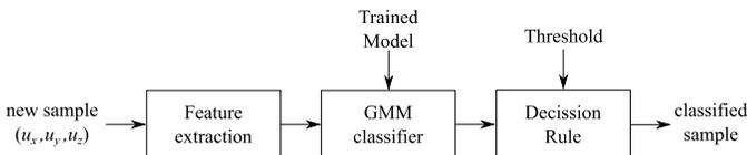
Figure 9. Flow chart of every fault detection test
