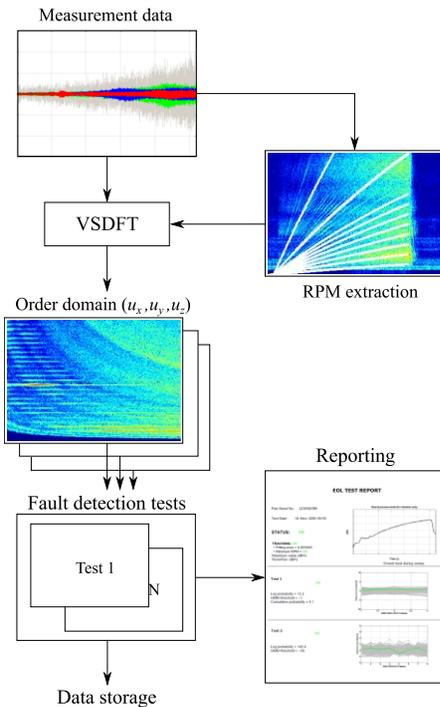
Figure 8. Flow chart of the EOL testing process
