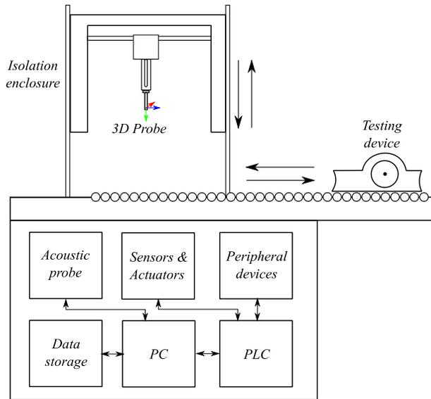
Figure 1. Sketch of the elements involved in the acoustic EOL system.
