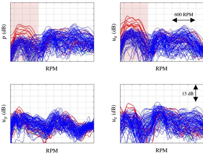
Figure 6. Comparison of the main motor order excitation level of regular (blue) and defective (red) units in terms of sound pressure (top left) and acoustic particle velocity in  $x$  (top right),  $y$  (bottom left) and  $z$  (bottom right) directions.
