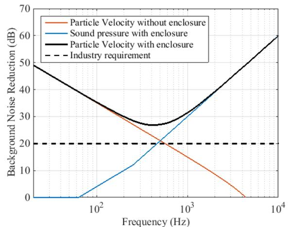
Figure 3. Background noise reduction levels that can be achieved with a sensor placed 0.01 m away from the testing object.
