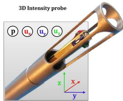
Figure 2. Picture of a 3D sound intensity probe.
