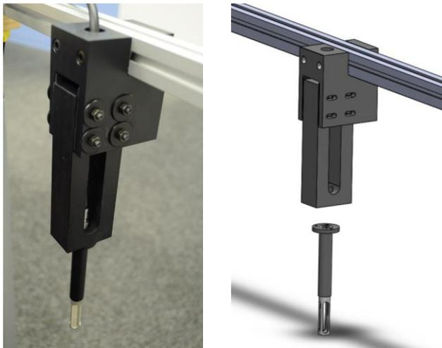
Figure 4. 3D probe attached (left) and detached (right) from the sensor holder.
