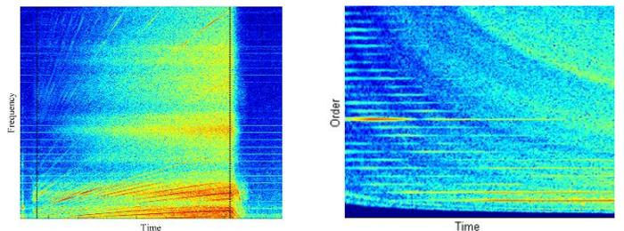
Figure 5. Time-frequency domain spectrogram during a run-up (left) and its equivalent order domain (right) computed using tach-less order tracking.
