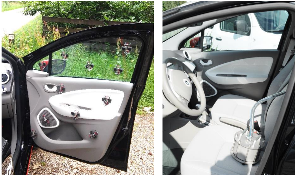
Figure 2: Pictures of the sensor attached to the front passenger door (left) and monopole source used for transfer path measurements (right).
