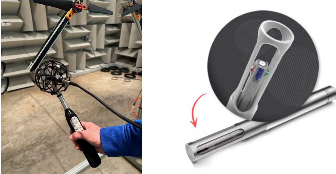
Figure 3: Scan&Paint 3D measurement in operation (left) and enlarged 3D sound intensity probe (right).
