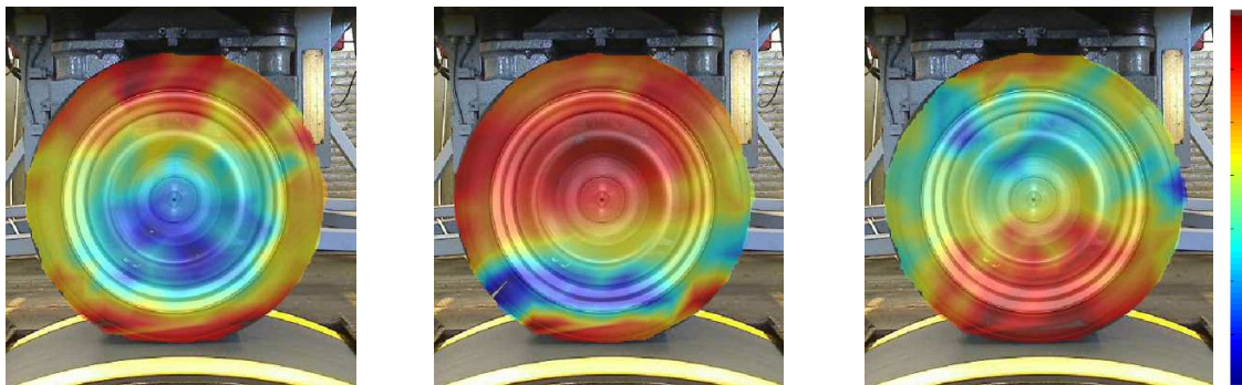
Figure 8. Measured vibration pattern for tyre 1 at 45 km/h. Left: 80 Hz. Middle: 375 Hz. Right: 425 Hz.
