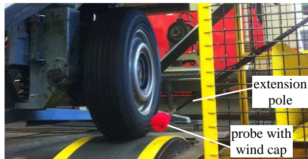
Figure 7. Tyre on the roller bench. The surface is scanned using an extension pole.
