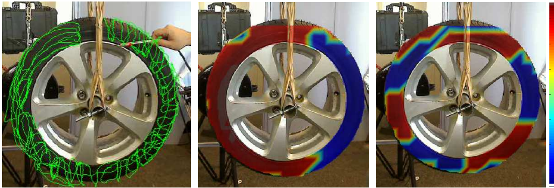
Figure 2. Side view. Left: Scanned path of the probe. Middle: ODS at 53Hz. Right: ODS at 199Hz.
