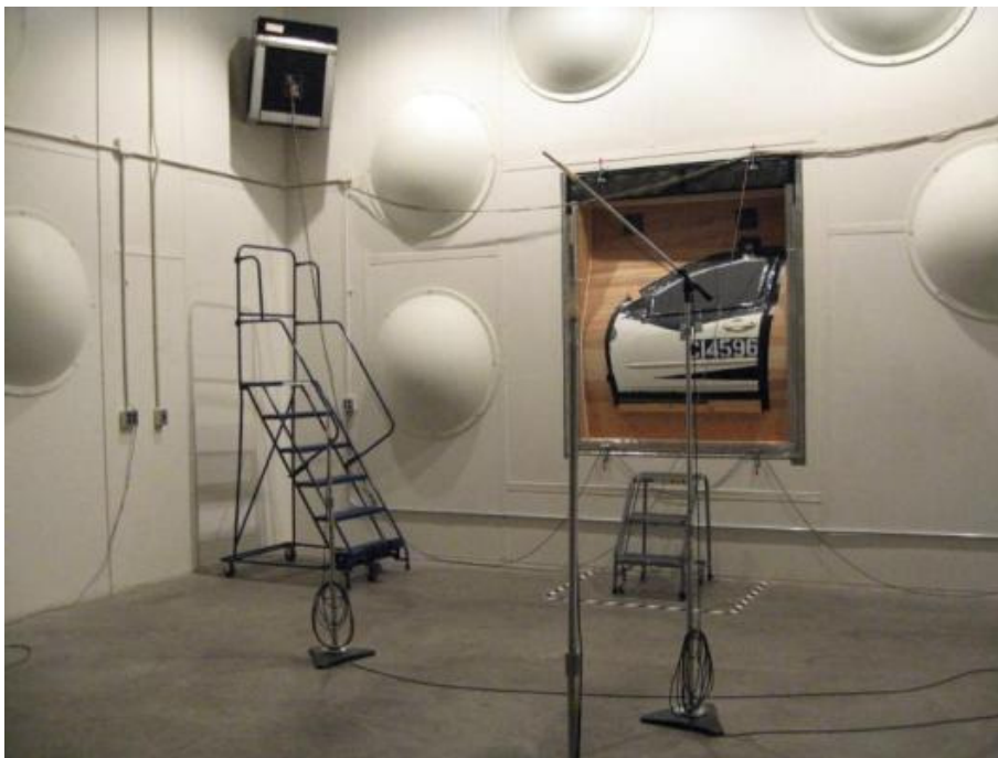
Fig. 19.4: Standard set up to measure the transmission loss of acoustic materials.
