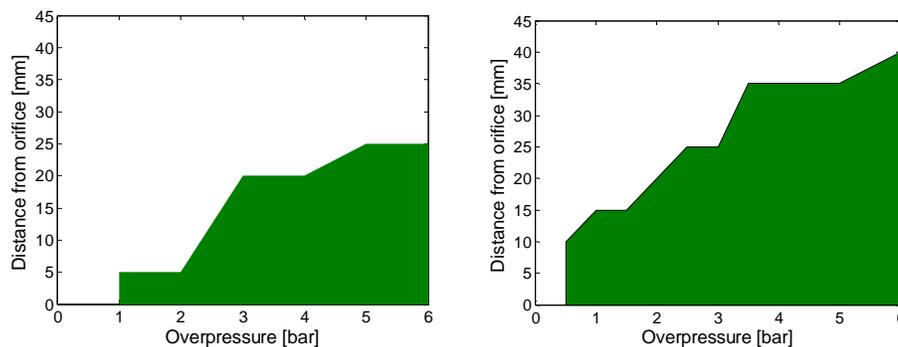
Fig. 18.12: Minimal measurement distance of a 3µm hole (left) and a 5µm hole (right).
