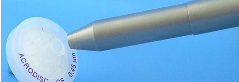
*Fig. 18.15: Leak testing of a filter.*
