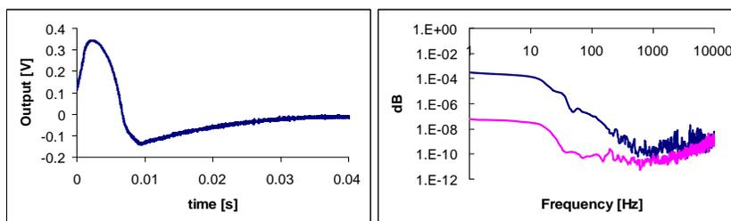
Fig. 18.7: Leak at 4 bar, leak size 3 micron. Left time signal, right representation in the frequency domain (Blue: leak signal, pink: no-leak signal).
