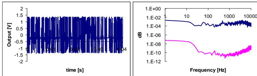
Fig. 18.6: Leak at 4 bar, leak size 10 micron. Left time signal, right representation in the frequency domain (Blue: leak signal, pink: no-leak signal).
