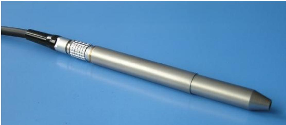
*Fig. 18.2: First prototype of the leak detection probe.*
