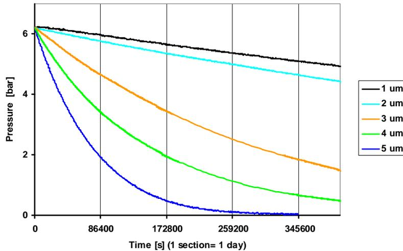
Fig. 18.10: Pressure decay measurements on five different orifices.
