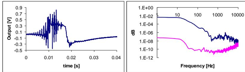
Fig. 18.8: Leak at 4 bar, leak size 5 micron. Left time signal, right representation in the frequency domain (Blue: leak signal, pink: no-leak signal).
