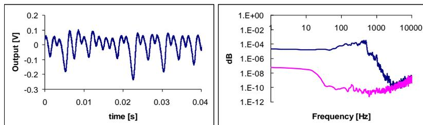
Fig. 18.4: Leak at 4 bar, leak size 3 micron. Left time signal, right representation in the frequency domain (Blue: leak signal, pink: no-leak signal).
