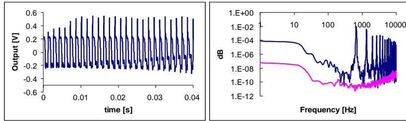
Fig. 18.5: Leak at 4 bar, leak size 5 micron. Left time signal, right representation in the frequency domain (Blue: leak signal, pink: no-leak signal).
