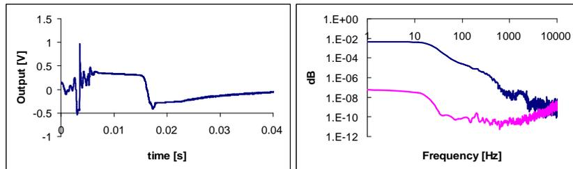
Fig. 18.9: Leak at 4 bar, leak size 10 micron. Left time signal, right representation in the frequency domain (Blue: leak signal, pink: no-leak signal).
