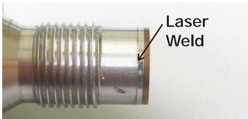
*Fig. 18.14: Leak testing of a laser weld.*
