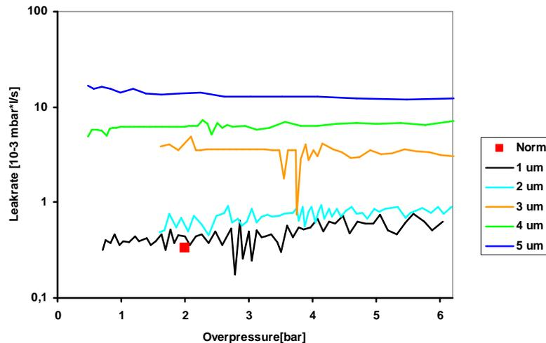
Fig. 18.11: Standard leak rate (at 1bar) calculated from pressure drop measurements.
