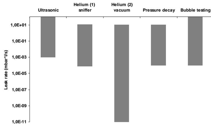
Fig. 18.3. Leak rate comparison of different methods.
