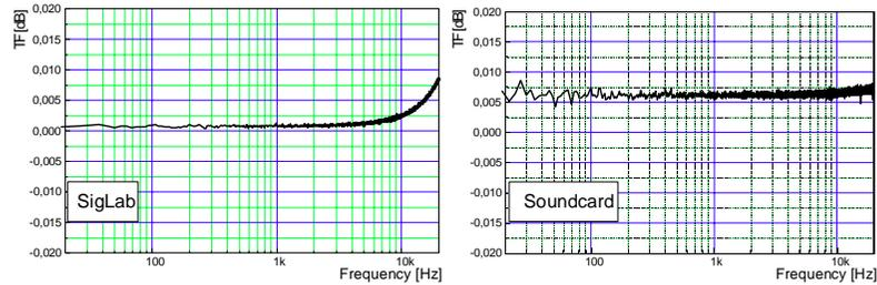
Fig. 16.4: Transfer function of two channels is measured to check the amplitude accuracy.
