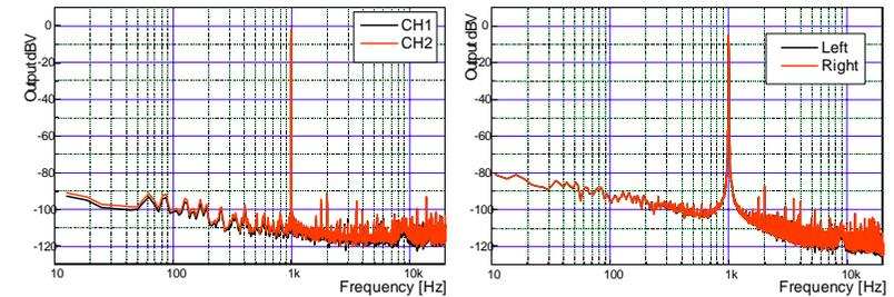
Fig. 16.2: A 1kHz sine wave is measured with (left) a Siglab analyser and (right) a low cost two stereo sound card.
