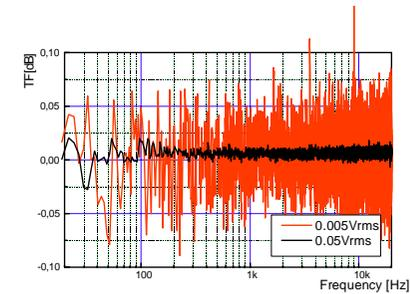
Fig. 16.5: Transfer function measured at 0.05V and 0.005V: if the input signal is too low the accuracy is low. (0.5V is full scale)
