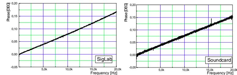
Fig. 16.3: Transfer function of two channels is measured to check the phase accuracy.
