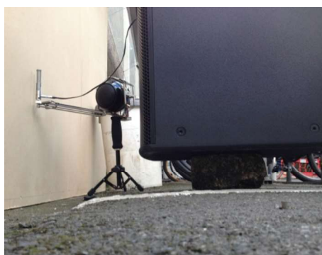
Figure 5: Mounting for the subwoofer had to be improvised. Here a concrete slab is used to lift it for the second row of measurements.
