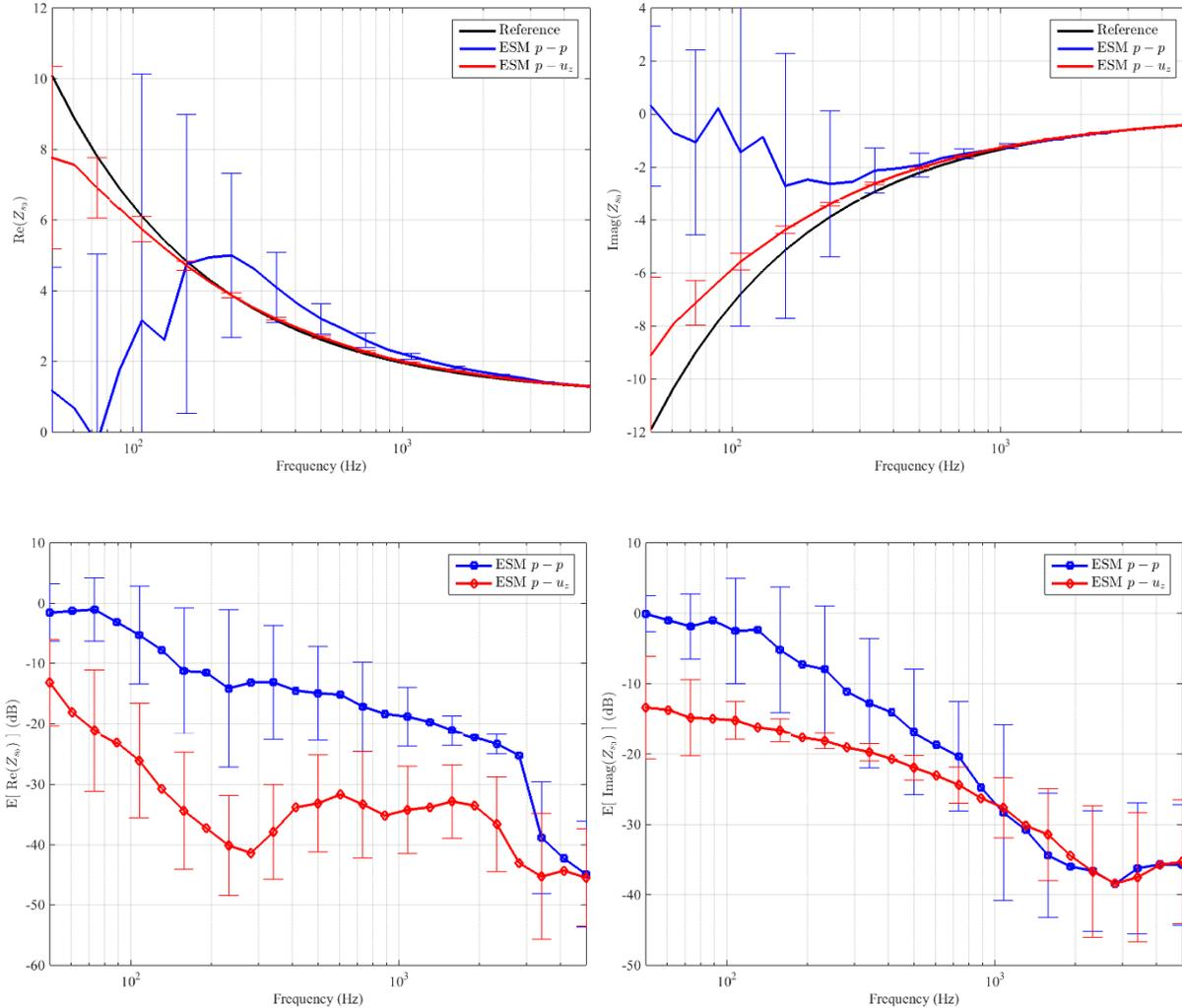
**Figure 3:** Normalized complex surface impedance: real part (top left), imaginary part (top right), relative error of real part estimation (bottom left) and relative error of the imaginary part estimation (bottom right). A confident interval of 95% is displayed with the same colors as the method used.
