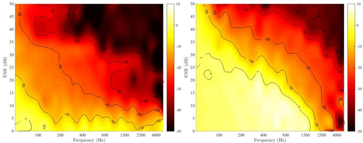
**Figure 5:** Reconstruction error of the surface impedance for variable SNR and frequencies with two different sensor configurations: single layer  $p$ - $u$  (left) and double layer  $p$ - $p$  (left).
