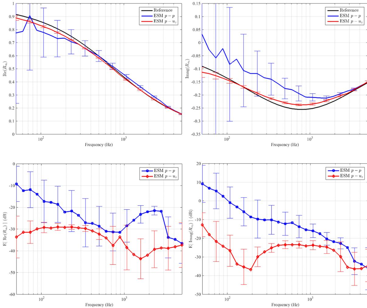
**Figure 4:** Normalized complex reflection coefficient: real part (top left), imaginary part (top right), relative error of real part estimation (bottom left) and relative error of the imaginary part estimation (bottom right). A confident interval of 95% is displayed with the same colors as the method used.
