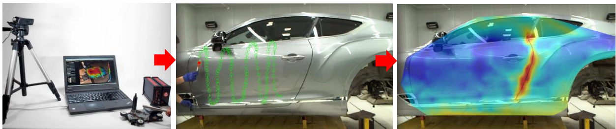
Figure 2: Illustration of the measurement equipment (left) and the basic steps of the Scan & Paint method: manual scan while recording a video (middle) and assessment of the sound maps (right).
