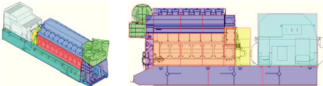
**Figure 1:** Left, partial sources division on a Wärtsilä V engine; Right, example of detail measurement segments for sound intensity scanning for a Wärtsilä in-line engine.
