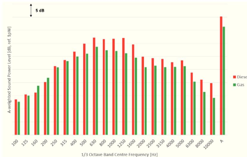
**Figure 5:** A-weighted sound power levels of a certain type of Wärtsilä dual-fuel gen-set running on diesel and gas modes.
