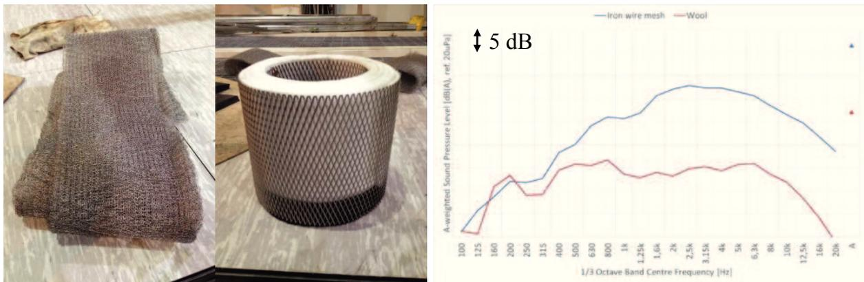
**Figure 9:** Noise level at 1 m distance away from the air wastegate silencer on a Wärtsilä engine with steel wire mesh and wool as the silencer absorption material.
