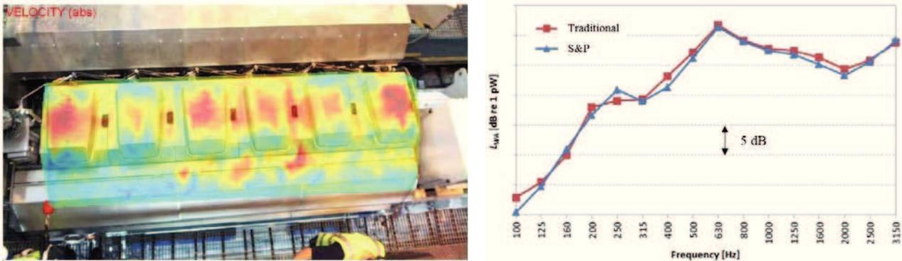
**Figure 3:** Left, particle velocity level of engine top part at a certain frequency band; Right, A-weighted sound power levels comparison between results from traditional and S&P probe.
