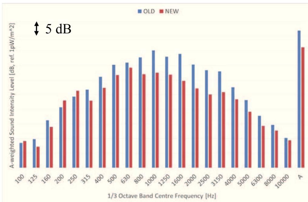
**Figure 10:** Manoeuvring side noise level comparison between old and new Wärtsilä 6L engines.
