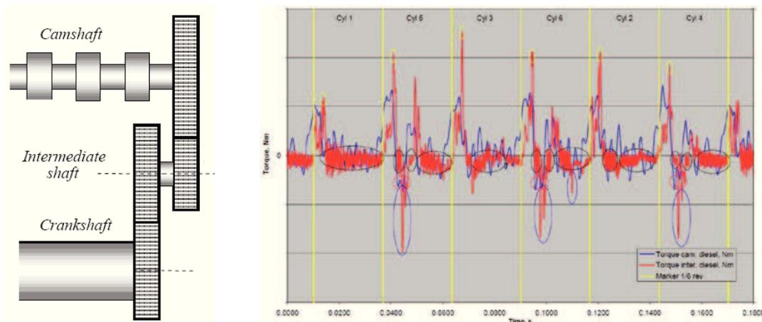
**Figure 6:** Camshaft and intermediate shaft torques measured on a Wärtsilä in-line engine with 6 cylinders. Red – intermediate shaft; Blue – camshaft.
