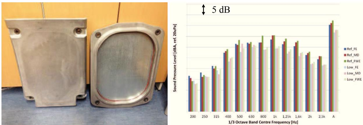
**Figure 8:** Left, cast aluminium and thin plate cover; Right, comparison of noise levels measured at 1 m distance away from the engine at free end (FE), middle part (MD) and flywheel end (FWE) between cast aluminium covers (Ref) and thin steel plate covers (Low).
