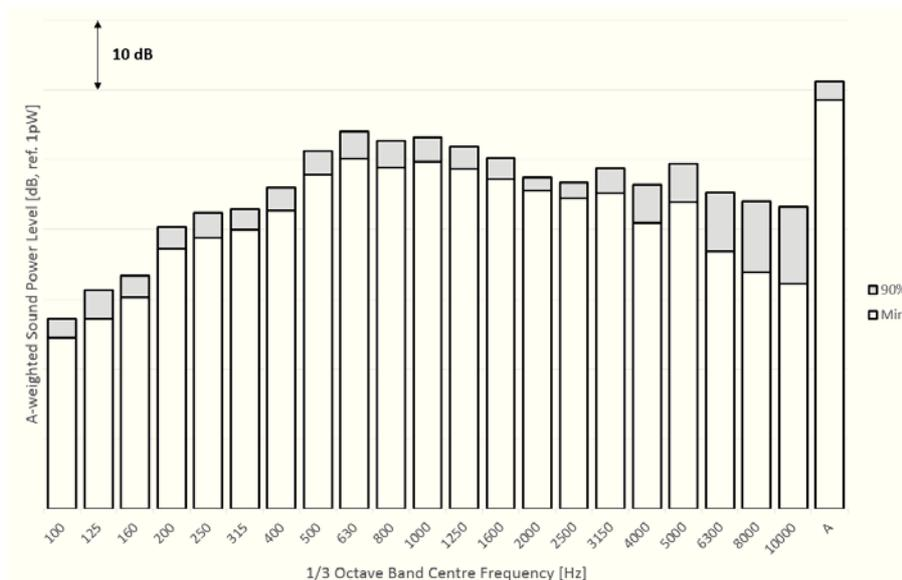
**Figure 4:** A-weighted sound power level of a certain type of Wärtisilä diesel engines. 90% of the measured engines have noise level within the grey area.
