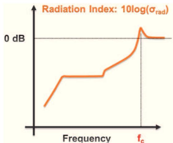
**Figure 7:** Demonstration of radiation index curve in frequency domain.
