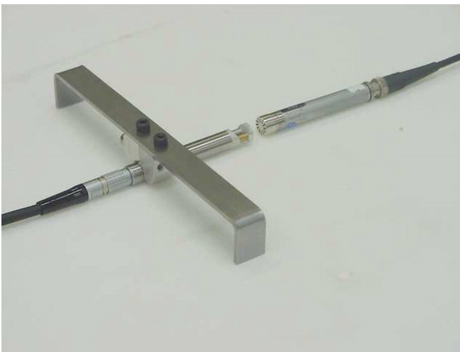
Fig. 12: The pu-impedance probe (left) and a reference pressure microphone (right) for verification purposes.
