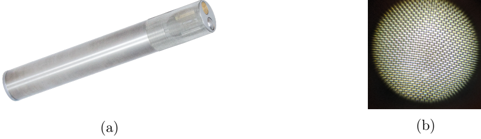
Figure 3.2: Steel mesh used in engineering applications. (a) PU Regular Probe covered in steel mesh, (b) Microscopic image of the steel mesh.
