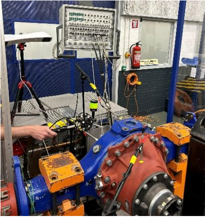
Figure 2. Scan&Paint 3D system used during the experimental testing campaign.
