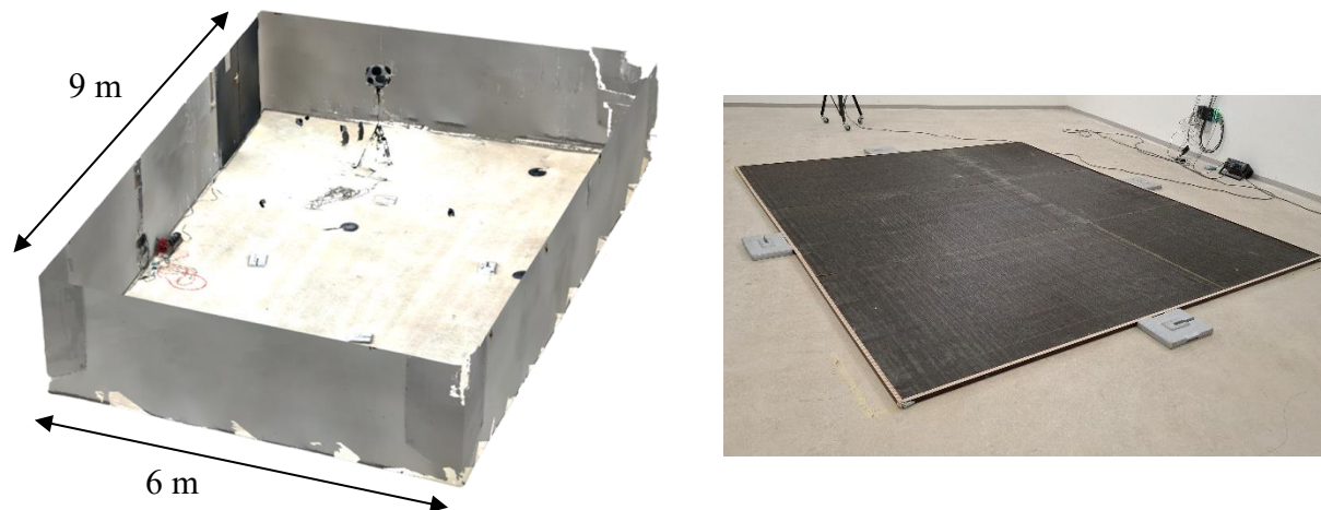
Figure 1: 3D model of the reverberant chamber (left) and photo of the sample used during ISO 354 tests (right).
