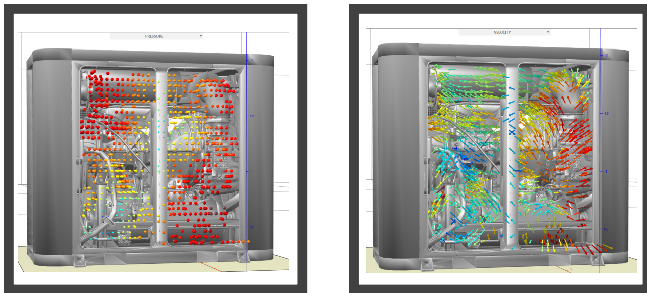
Figure 4: Comparison between Sound Pressure (left) and Particle Velocity (right) for 100-140Hz, covering the 3rd tone
