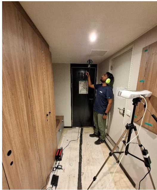
Figure 2: Performing a Scan & Paint 3D measurement on a partition surface
