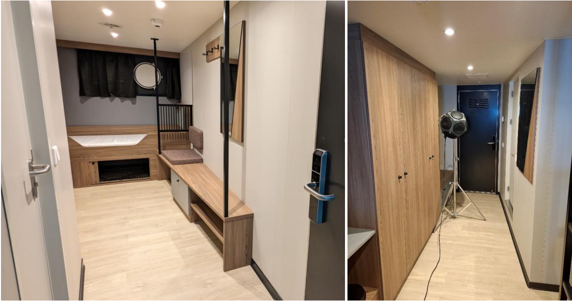
Figure 1: Measurement setup in an finished (a) accommodation space with (b) dodecahedral sound source
