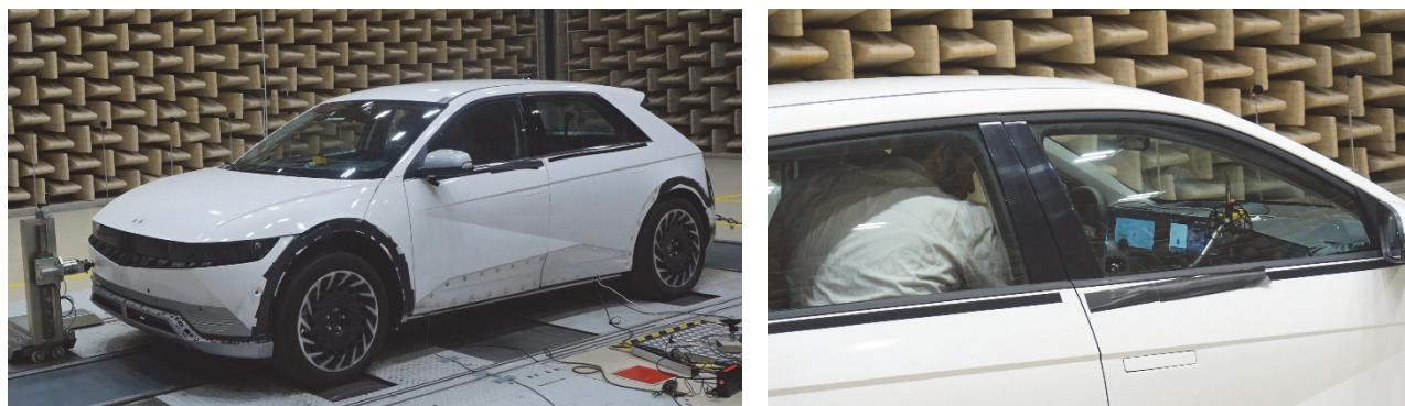
**Figure 3:** Figure 3. on semi-anechoic vehicle dyno constant speed measurement at 80kph and 100kph (left) and example of the sound intensity field measurement inside of vehicle (right).
