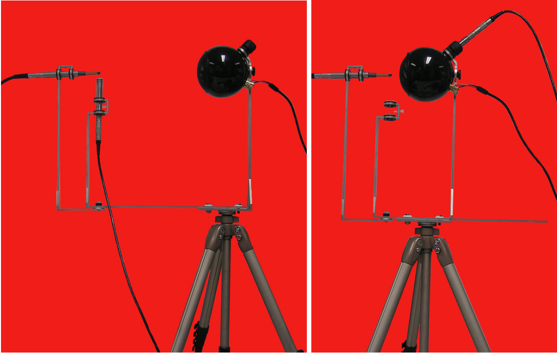
Fig. 4A.11: The new small sphere calibration set up.
