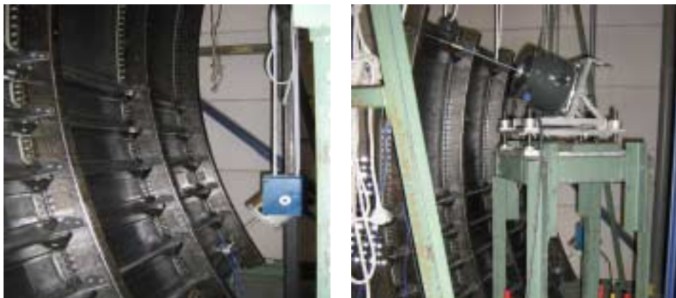
Figure 2 Shaker 1 (left) and shaker 2 (right) coupled to the panel
