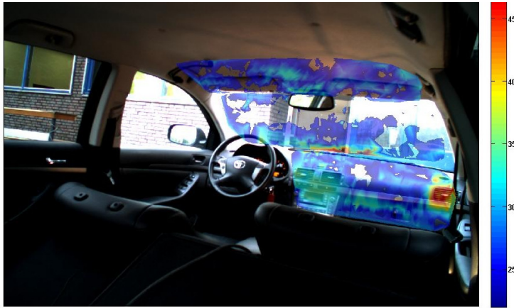
Fig. 5: Velocity distribution inside a car (400Hz)
