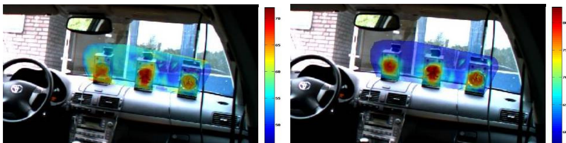
Fig. 6: Colour map of three speakers (white noise input). Left: 55-143hz. Right: 800-1500Hz
