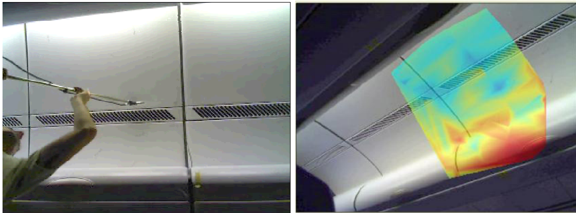
Fig. 3: Left: The surface of an aircraft luggage compartment. Right: Velocity (10-1000Hz). The total measuring plus processing time was in the order of ten minutes.
